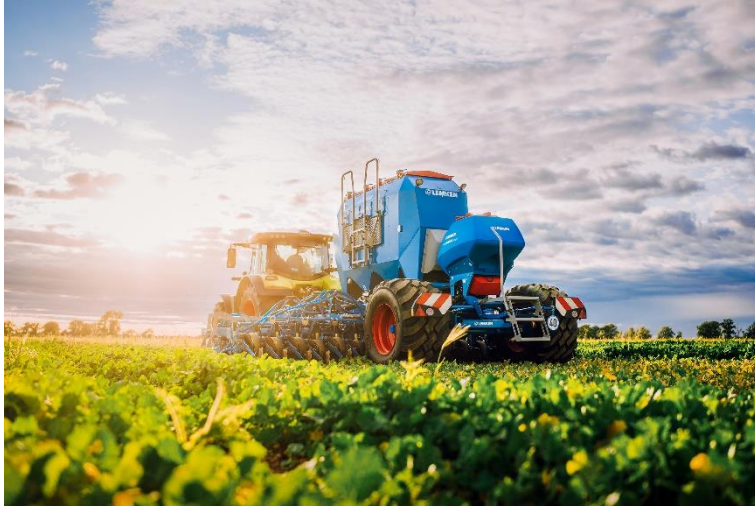
Image 1: The LEMKEN Solitair NT has been specially designed for conservation tillage systems.
